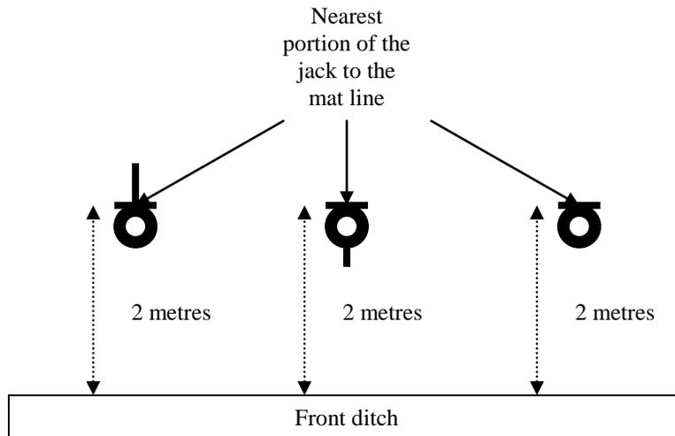
B.3.2 Position of the jack alongside a 2-metre measuring device
